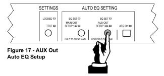
At step 4, once the **AEQ ON** indicator has illuminated, the Auto EQ for all connected EVO Loudspeakers can be listened to simultaneously. *See Testing Auto EQ*.
